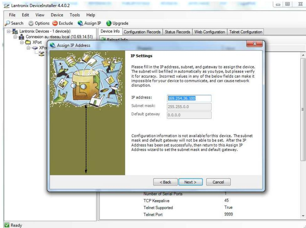
When the assignment is finished, click on "Finish" button and the AGATH IP control box is configured.
